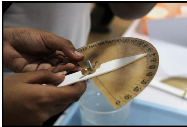
A protractor with tactile markings, which is used by visually impaired students
