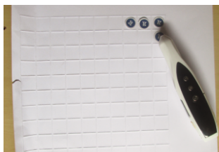
Image of an audio labeller and labels on a tactile graph paper
