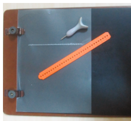
Image of a tactile drawing paper and a rubber mat on a board, with a tactile ruler and stylus
